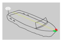
**Sidelights** shall be positioned at a height above the upper most continuous deck not greater than  $\frac{3}{4}$  the height of the masthead light (Annex I – 2(g)).
