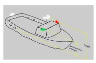
In cases where the sidelights are in a combined lantern they shall be placed not less than 1 meter below the masthead light or all-round white light (Annex I – 2(h)).
