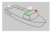
It may be displaced if not practical, but **sidelights** must be combined in one lantern and placed on the fore and aft centerline of the vessel (Rule 23(c)(i)).
