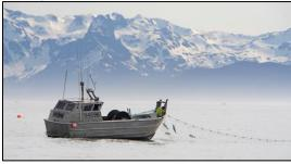
Gillnet vessels are typically 25 to 32 feet long. They are easily recognized by the hydraulic-powered drum onto which the net is rolled. The drum can be located on the stern or bow of the vessel. Crew size is 2-4 POB. Target species is typically salmon.
