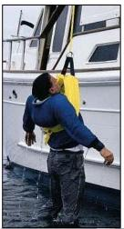
The Lifesling3 Overboard Rescue System bearing CG Approval #160.050 may replace a Type IV 24-inch ring life buoy provided the vessel has a lifting point 10 feet above the deck, the device is stowed per the instructions, the crew is familiar with the operation of the device and a manual is on board the vessel.
