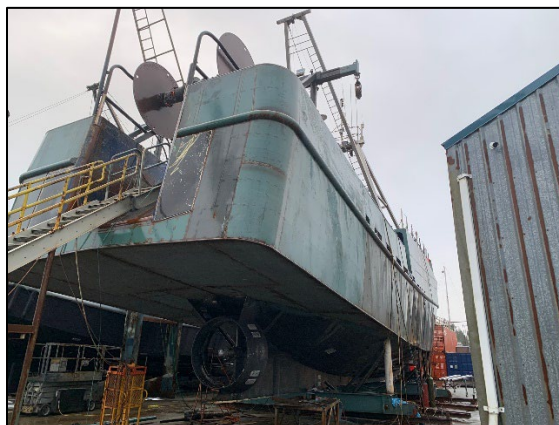
Former Gulf Shrimper has their stern squared off to better suit trawling in the North Pacific
