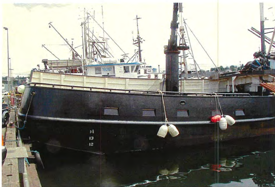
High bulwarks help protect the crew from the weather
