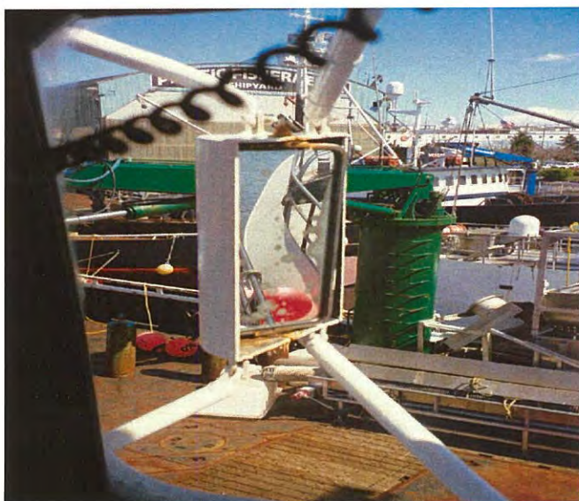
A truck mirror gives a good view of the pot line
