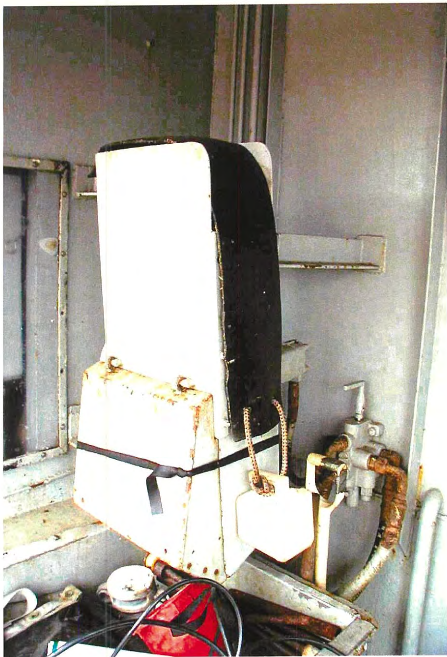
Bait Chopper Cover Guards can save fingers!
