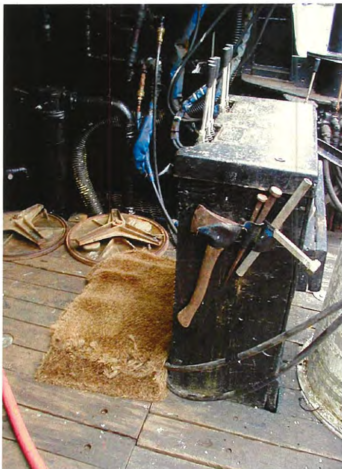
Fiber mats can prevent falls in slippery areas
