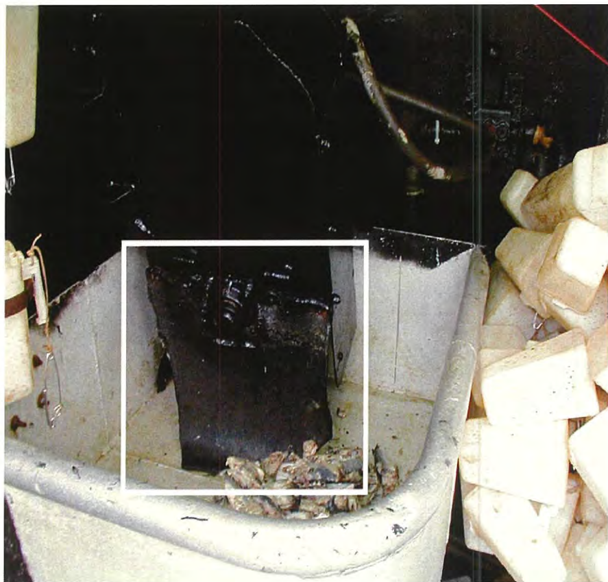
A bait chopper bottom guard protects the crew's hands as they scoop out bait
