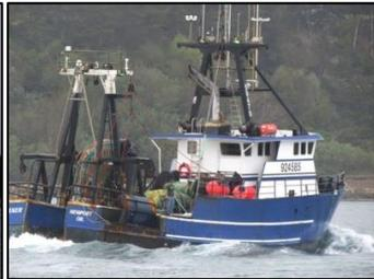
**Side trawlers** have the trawl deployed over the side.
