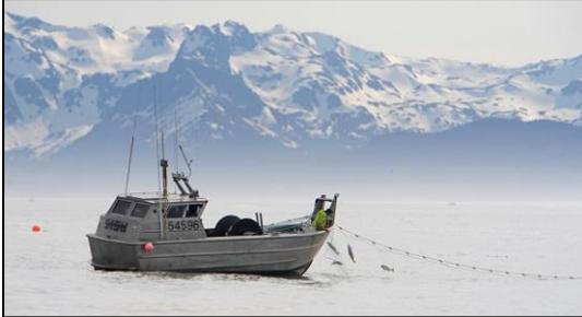
Gillnet vessels are typically 25 to 32 feet long. They are easily recognized by the hydraulic-powered drum onto which the net is rolled. The drum can be located on the stern or bow of the vessel. Crew size is 2-4 POB. Target species is typically salmon.
