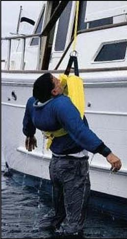
The Lifesling3 Overboard Rescue System bearing CG Approval #160.050 may replace a Type IV 24-inch ring life buoy provided the vessel has a lifting point 10 feet above the deck, the device is stowed per the instructions, the crew is familiar with the operation of the device and a manual is on board the vessel.
