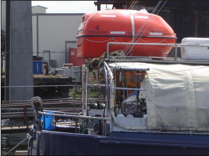
Although Ovatek rigid liferafts do not require annual servicing, the equipment packs inside and the HRU does require regular maintenance. Special attention should be paid to expiration dates of distress signals, water & food rations and batteries.
