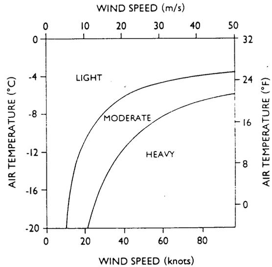
Icing conditions for vessels heading into or abeam of the wind for water temperatures of +7°C (45°F)
