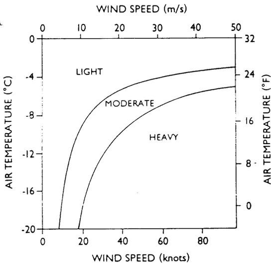
Icing conditions for vessels heading into or abeam of the wind for water temperatures of +5°C (41°F)
