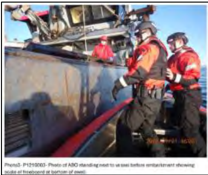
Example: (L) High freeboard; (R) COMAR MARK 1 Pilot Ladder
